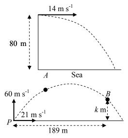
The displacement of point *B* from *P* is 189  $\vec{i} + k \vec{j}$  m.
